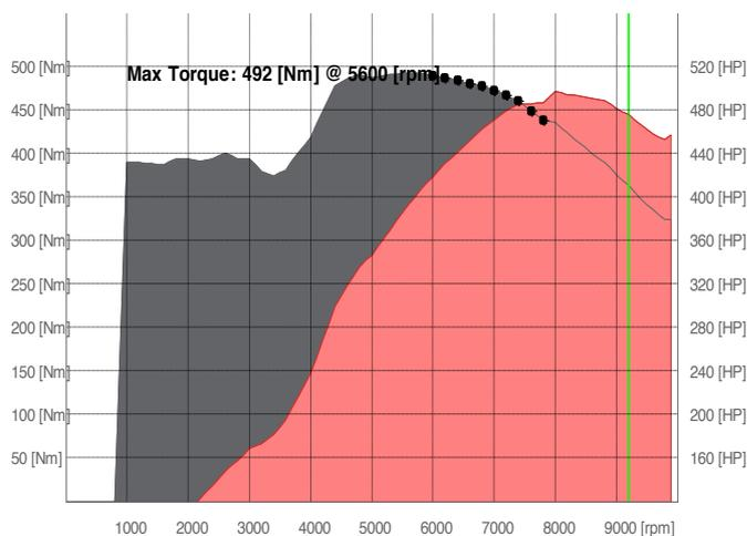
**Figure 5: option 2; a 4-litre V8 for a 2014 LMP**
