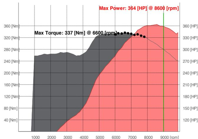
**Figure 4: a 2.8 litre 6 cylinder engine for a 2014 LMP**
